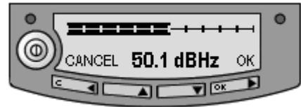
The EXPLORER™ 500 now tries to establish a connection to the BGAN network. The display shows the progress as follows:
