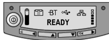
The Main screen also shows icons for any interfaces that are turned on. In this example, all interfaces (Phone/Fax, Bluetooth, USB and LAN) are turned on.
