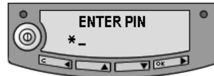
To correct an entered digit, press **C** to go back and use the ▲ and ▼ buttons again.
