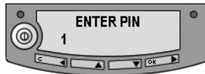
3. Press **OK** to go to the next digit. When **OK** is pressed, the previous digit is indicated by a \*.
