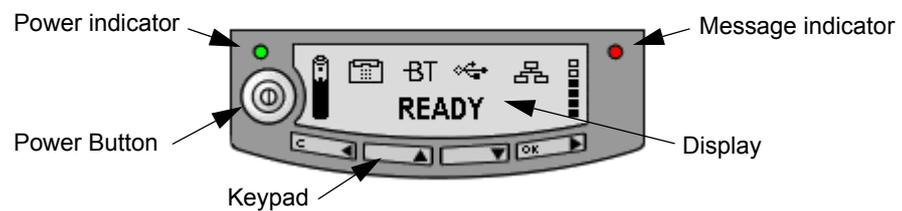
For information on how to use the keypad and display, and for an overview of the display menu system, see *Using the display and keypad* on page 30.
