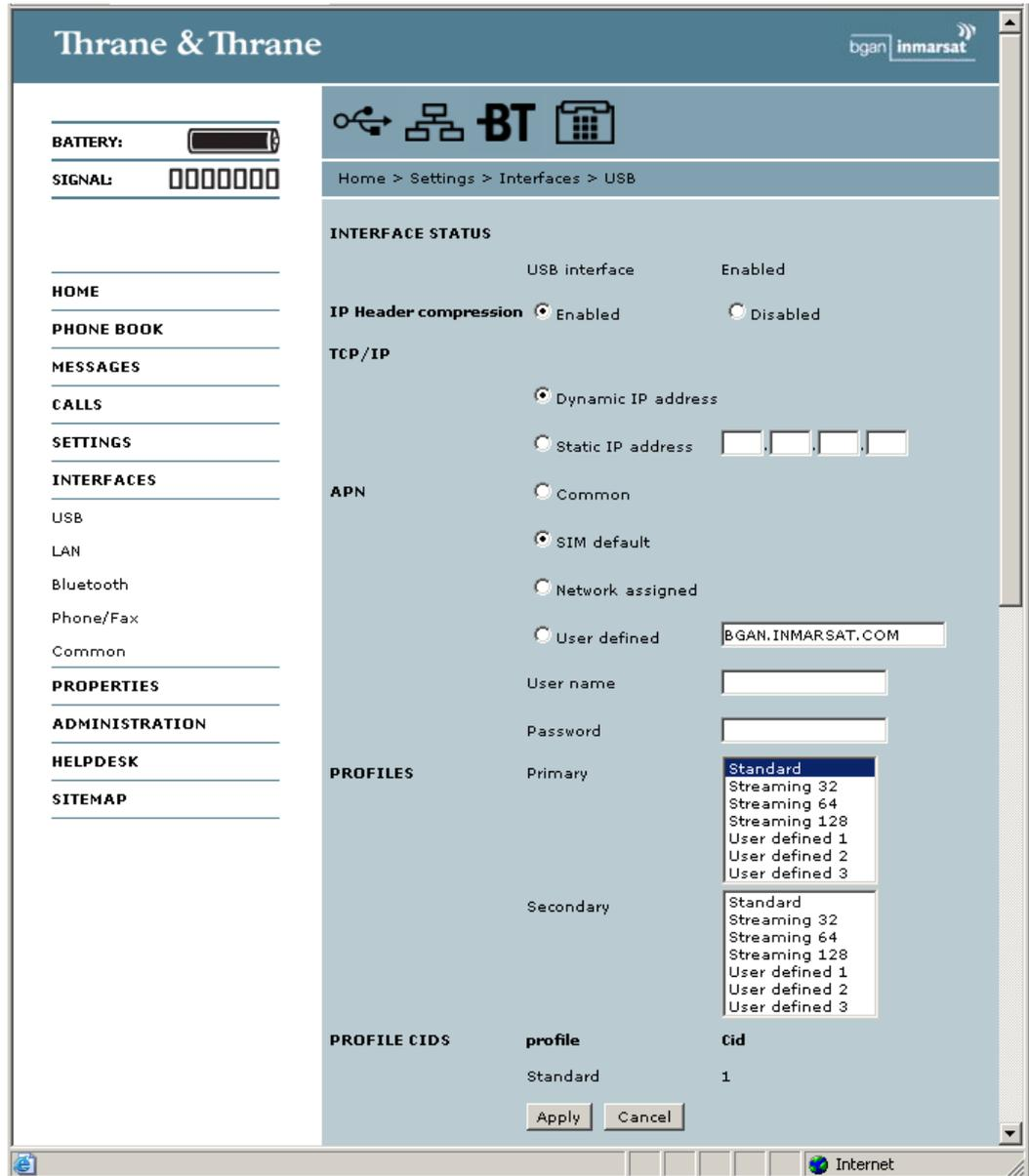
2. Under **TCP/IP**, select whether your computer uses a **Dynamic IP address** or a **Static IP address**. If you are using a static IP address, type in the address.
