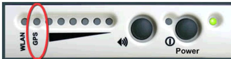
Now leave the terminal to acquire a GPS fix. This may take a few minutes. Once the GPS fix has been acquired the GPS LED will turn solid green.
