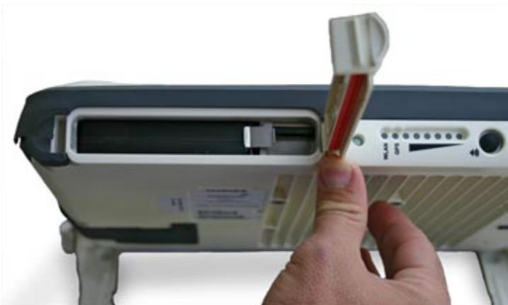
3. Push the button on the left-hand side of the USIM/SIM card holder. This releases the holder from its slot.
