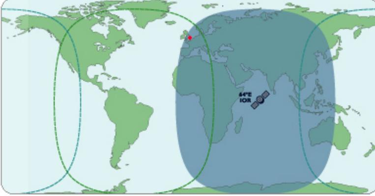
Recommended: Antenna angle: 8° Compass direction: ESE (113°)
