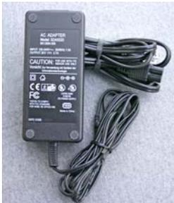
2. Insert the power adapter output connector to the DC Power Input Jack on the back of the Terminal. Insert the plug end into any AC outlet between 100 and 240 VAC.
