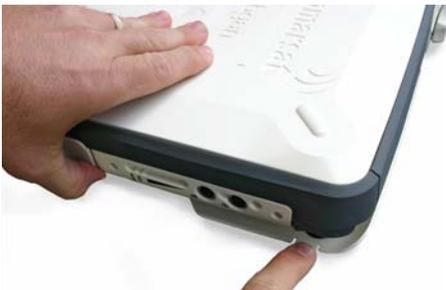
3. Pull out the front stabilizer. Lay the Terminal back on the flat surface.
