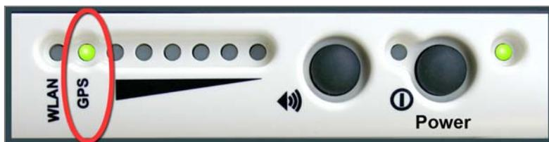
The GPS unit in the Satellite Terminal will attempt to get a 3D fix each time the unit powers up. The GPS LED indicates the state of the GPS fix. See **Obtaining a GPS Fix** section.
