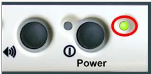
The Battery LED indicates battery status. The indicators are different when the Terminal is on DC power as opposed to on battery power.
