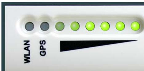
These six, two-color LEDs have significance for two events: System Power-Up/Boot-Up and Antenna Pointing.
