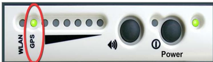
3. Monitor either the BGAN LaunchPad GPS indicator or the Terminal's GPS LED for the quality of the GPS fix. This may take a few minutes. Once the GPS fix has been acquired the GPS LED will turn solid green.
