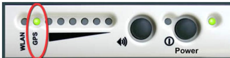
**Note:** If the GPS indicator light is solid red, the GPS receiver is faulty. Contact your Service Provider.
