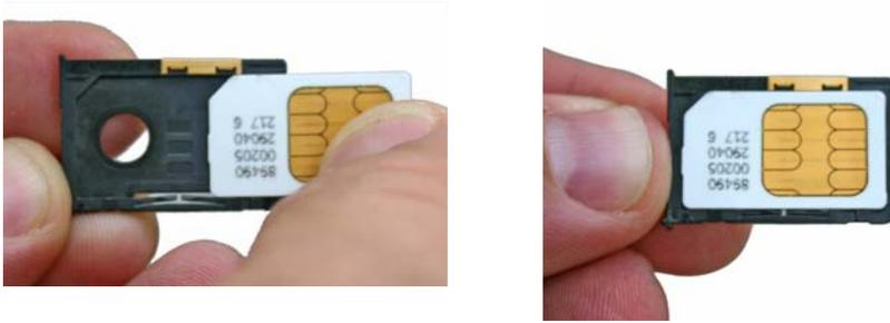
5. With the card in place, orient the holder with the card's gold shield facing down. Place the holder back in its slot in the MT.
